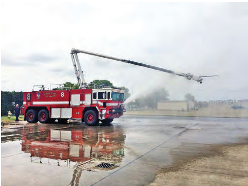
Oshkosh airfield fire appliance in action. The elevating turret with lance attachment can be seen and the front fender spray is being deployed.
